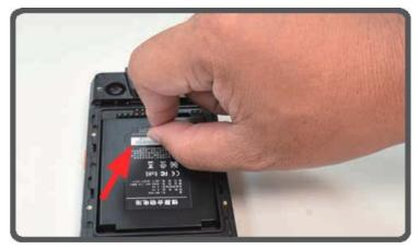
**Step 4:** Insert the battery make sure the battery pins are connected to the probe
